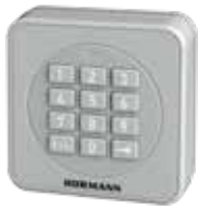
Radio code switch FCT 3 BS 3 functions, with illuminated buttons, recessed or surface-mounted fitting possible, plastic housing in Light grey RAL 7040 (also available with 10 functions and hinged cover, painted in White aluminium RAL 9006)
